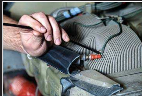
Inspecting cylinder in aircraft motor with VSA2-1M
